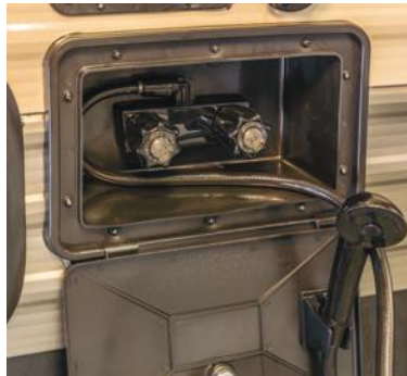
Outside Shower with Hot and Cold Water
