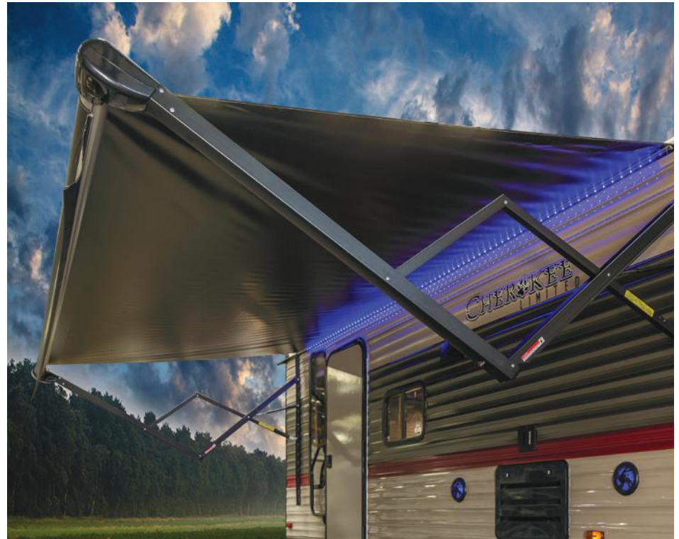
Power Awning with Blue Led Strip Lighting
